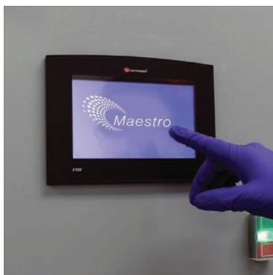
Backlit touch screen controls for monitoring and reporting analyses, configuring system alarms, and exporting data.
